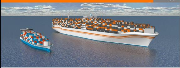
A larger ship will in most cases offer greater transport efficiency – "Efficiency of Scale" effect. A larger ship can transport more cargo at the same speed with less power per cargo unit. Limitations may be met in port handling.
