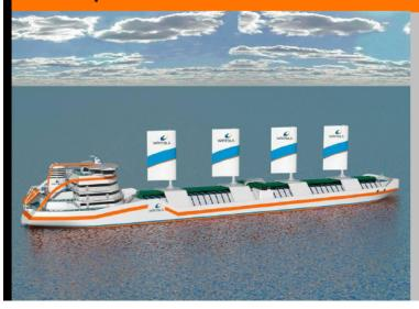
Wing-shaped sails installed on the deck or a kite attached to the bow of the ship use wind energy for added forward thrust. Static sails made of composite material and fabric sails are possible.
