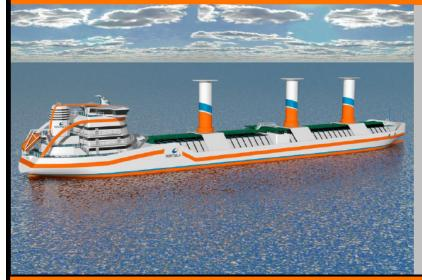
Spinning vertical rotors installed on the ship convert wind power into thrust in the perpendicular direction of the wind, utilising the Magnus effect. This means that in side wind conditions the ship will benefit from the added thrust.
