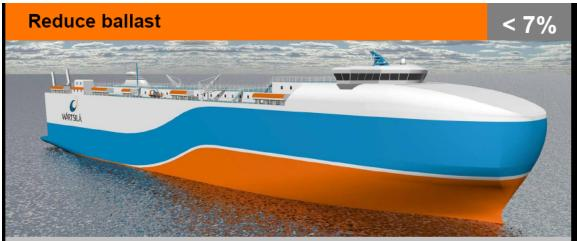
Minimising the use of ballast (and other unnecessary weight) results in lighter displacement and thus lower resistance. The resistance is more or less directly proportional to the displacement of the vessel. However there must be enough ballast to immerse the propeller in the water, and provide sufficient stability (safety) and acceptable sea keeping behaviour (slamming).
