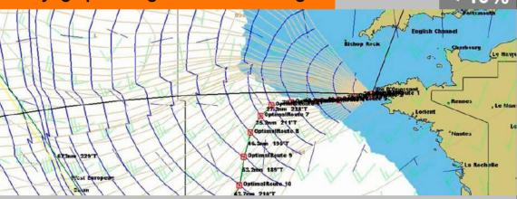
The purpose of weather routing is to find the optimum route for long distance voyages, where the shortest route is not always the fastest. The basic idea is to use updated weather forecast data and choose the optimal route through calm areas or areas that have the most downwind tracks. The best systems also take into account the currents, and try to take maximum advantage of these. This track information can be imported to the navigation system.
