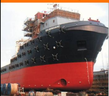
Modern hull coatings have a smoother and harder surface finish, resulting in reduced friction. Since typically some 50-80% of resistance is friction, better coatings can result in lower total resistance.
