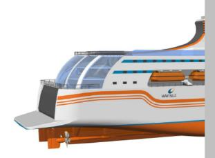
A ducktail is basically a lengthening of the aft ship. It is usually 3-6 meter long. The basic idea is to lengthen the effective waterline and make the wetted transom smaller. This has a positive effect on the resistance of the ship. In some cases the best results are achieved when a ducktail is used together with an interceptor.
