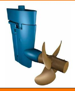
The rudder has drag in the order of 5% of ship resistance. This can be reduced by 50% by changing the rudder profile and the propeller. Designing these together with a rudder bulb will give additional benefits. This system is called the Energopac® system.
